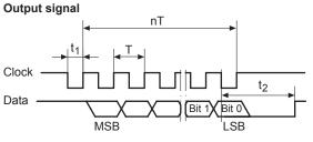
$T = 0.5...10 \ \mu s$   $t_1 = 0.25...5 \ \mu s$   $t_2 = 20 \pm 2 \ \mu s$  f max. = 2 MHz
